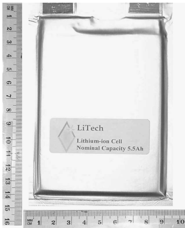
Fig. 1. Picture of a 5.5 Ah lithium-ion cell made with carbon fiber composite anode, LiCoO 2 cathode, and 1.4 M LiPF 6 in EC/EMC (1:3, v/v).
